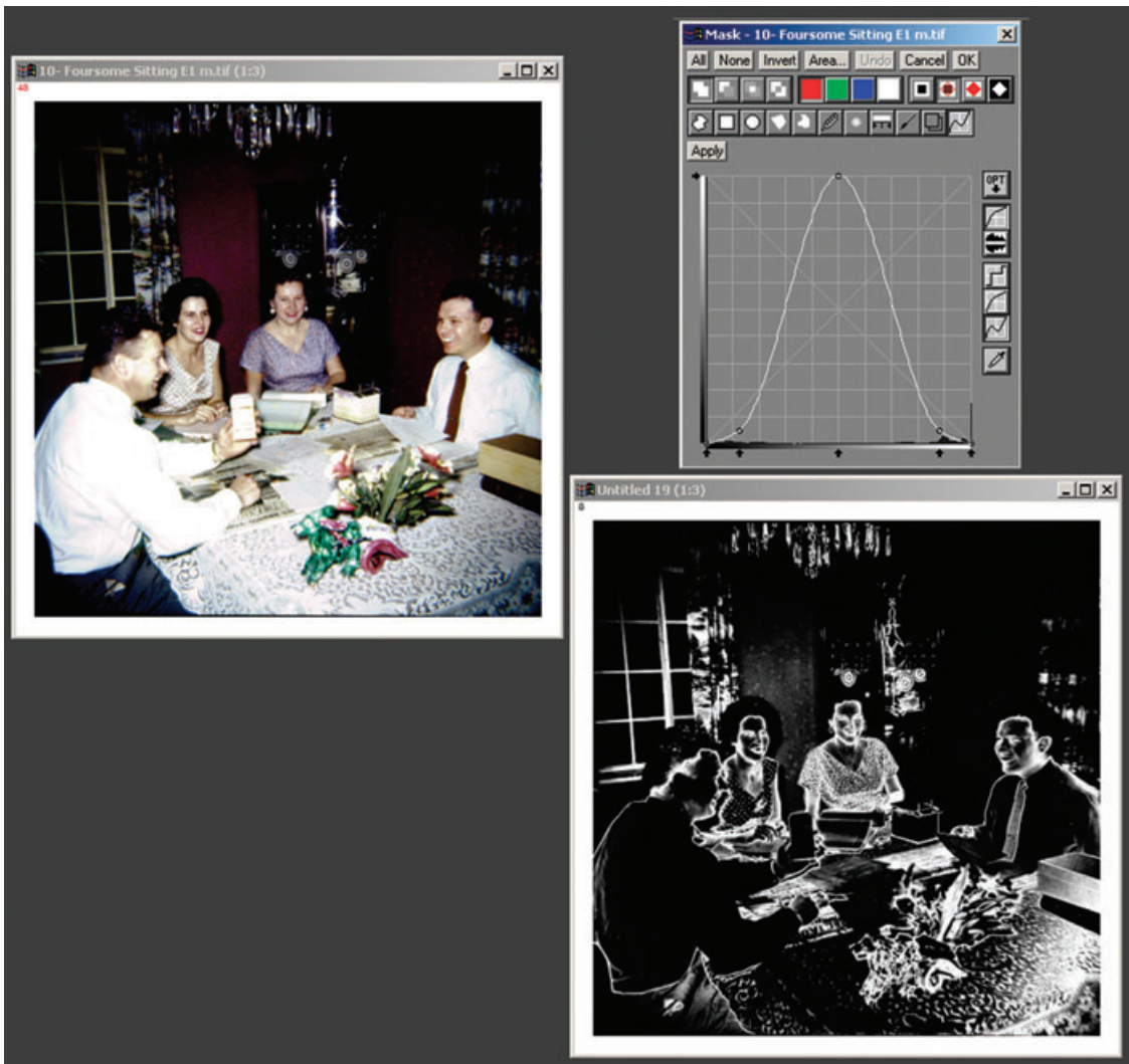
Fig. 3-5 Picture Window has some very powerful mask-making tools. The Mask Brightness Curve, for example, is much more flexible and useful than Photoshop's crude Color Range tool. Here I used the Curve to create a mask (lower right) that selected the midtones of the photograph in the upper left and smoothly faded out toward the whites and blacks. You can create very complex masks by using several of the masking tools in combination.
